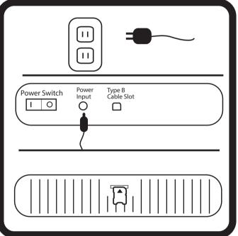
Plug the power supply into the wall and then into the printer. Insert the SD card into the SD slot on the left side of the printer. Turn on the machine via the on/off switch on the back.
