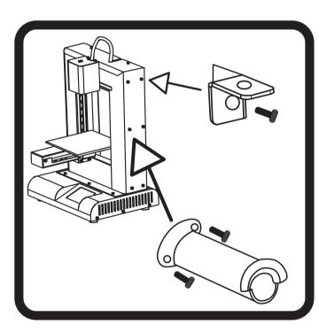
Screw in the spool holder and filament guide into the printer using the screws already on the body of the printer. These need to be placed on the same side of the printer. The long side of the filament guide should be perpendicular to the body of the printer.
