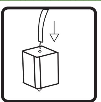
Insert the filament into the extruder hole, located on top of the extruder head. Push the filament in until it won't go any further, the printer will grab onto it once printing begins.
