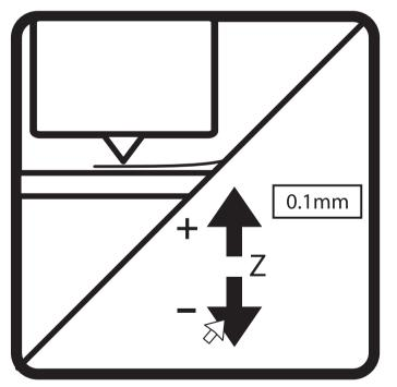
Calibrate print height and level (see calibration guide).
