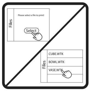
Touch the LCD screen and press the scan button. A list of all the files on the SD card will be shown. Select a file to print and the printer will begin to warm up then begin printing. (Optional) Apply a thin layer of glue from a standard glue stick or a spritz of hairspray onto the print plate to further help the print adhere.
