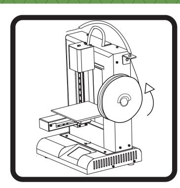
Attach the filament roll to the spool holder so that the printer will pull the roll counterclockwise. Insert the filament through the filament guide and filament guide tube.
