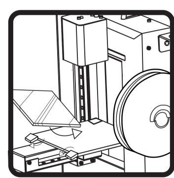
The front clips located on the print bed swivel outwards for easy access. Slide the glass plate under the clips located in the back. Then swing the front clips around to secure the glass plate in place. Clips may fit tightly, take care not to injure yourself during installation of glass plate. (Optional) Apply the included blue tape to the glass before sliding it into place, doing so will increase print adhesion.
