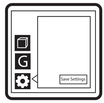
Once the platform has fully descended a number will appear next to the "Z:" display located at the bottom of the panel. Simply click the "Save Settings" button next to the "Z:" display and your printer will use that as its default height for all future prints. (Please note that whenever your remove or adjust your platform for whatever reason, you may need to recalibrate your printer)
