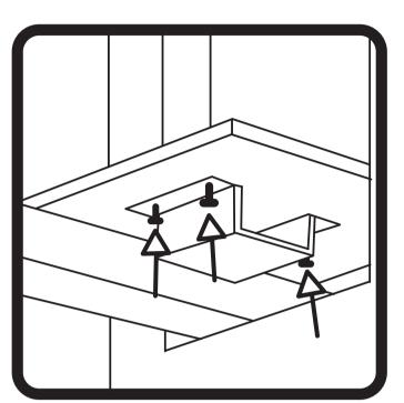
Move the extruder over each of the corners of the print bed. Use the included allen wrench to loosen/tighten each of the three springs located under the print plate to bring each corner of the print bed closer to the extruder.
