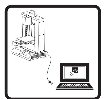
Connect the printer to your computer via the USB cable. Then in the Germinate software click the USB symbol to connect the printer and software.
