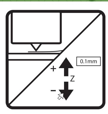
Increase the height via the on-screen controls. Next to the Z +/- arrows buttons that are at the top of the panel will be "continue" "Lock" and "Unlock." Select "continue" and set it to 0.1mm. Click the Z+ arrow to increase the print plate's height and use a business card to gauge the distance between the platforms height and the printing plate until it is no longer able to slide freely between them. (The card should be able to slide between the plate and nozzle with minimal resistance.)
