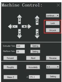
4.3.9.5 Set the nozzle temperature: input the target temperature and click "Setting", and the nozzle begins heating. For PLA material, the recommended temperature is 220-230 °C and for ABS material, the recommended temperature is 230-240 °C.
