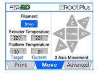
3.1.13 If the printing is suspended for a long time, to avoid clogging next time, take out the filament inside the extruder. After the extruder temperature rises to the set value, click "Reverse". After the filament returns completely, take it out, and click "Stop".
