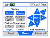
3.1.12 After the extruder temperature rises to the set value, click "Forward", and insert the prepared filament into the extruder's feed port till the extruder catch the filament. After a few seconds, you can see fine filament out of the nozzle. Click "Stop", and the extruder stops. At this moment, the interface is as shown in the following figure.
