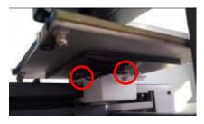
3.1.20 After determining the direction of Y-axis, move the platform to make the extruder in the center. Click "X-" or "X+" to move it left and right.
