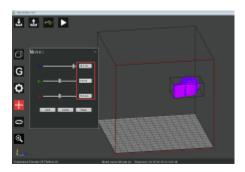
4.3.10.4 After the model is rotated, scaled or moved, if you want to move the model to the center of the platform, click "Land" and " center" or click "Reset" to return to the original state of model printing.
