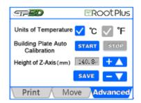
3.1.23 To modify Z-axis height, you can also directly click the display frame, and a numeric keypad will pop up. Input the height value(mm) you want, click "OK" to return to the interface "Advanced", and click "SAVE".
