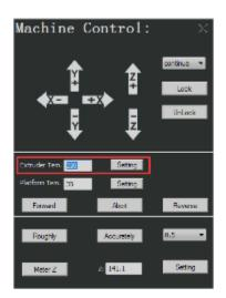
4.3.9.6 Set the platform temperature: directly input the target temperature and click "Setting", and the platform begins heating.
