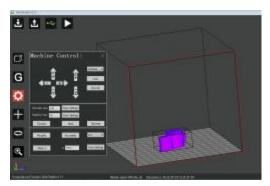
4.3.9.2 GP3D Root Plus control includes three parts: movement control"1", temperature control "2" and Z-axis height setting "3", as shown below.
