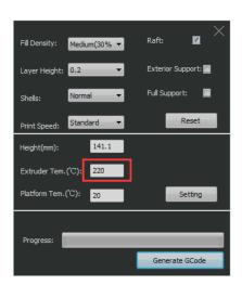
4.3.8.17 Set the platform temperature: directly input the temperature in the dialog box and click "Setting". For PLA material, the recommended temperature is 40  $^{\circ}$ C or below and for ABS material, the recommended temperature is 80-100  $^{\circ}$ C according to the size of the model.
