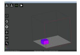
4.4.2 Select the model with the left mouse button, click the left menu button to move the model to the center of the platform, and you can click "center", as shown below.
