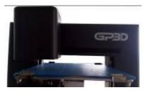
3.1.18 Click "Y-" or "Y+" to move the platform back and forth to observe whether the distance between the nozzle and the platform is equal all the time.
