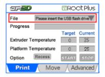
3.1.3 After the USB flash drive is inserted, the inverted triangle turns blue, and the pull-down menu displays the file to be printed.
