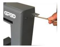
2.2.4 Fixation of hotbed panel: fix the hotbed panel on the build plate with four clamps.
