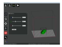
4.3.11.3 To operate one of several models, first select the model with the left mouse button, and then the model can be rotated, as shown below.
