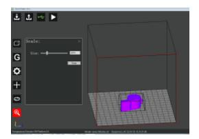
4.3.12.2 Move the slider with the mouse or input directly the zoom scale in the dialog.
