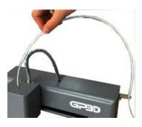
2.2.8 Power on: plug the output end of the power adapter into the power interface on the GP3D Root Plus.
