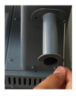
2.2.3 Assembly of filament card: take out the screw at the back of the upper right side of the GP3D Root Plus and fix the filament card with the screw.
