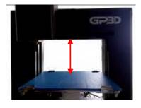
3.1.19 If the distance is equal, enter the next step. If not, adjust the screw fixing the platform till it is equal.
