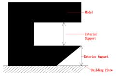
4.3.8.13 In print parameter settings, check Exterior support and Full support, as shown below.
