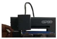
4.3.9.12 Click "Meter Z", and the GP3D Root Plus automatically starts measuring. You can see the increase of the figure in the dialog after "Z:". After the measuring is complete, click "Setting" to complete the measuring of Z-axis height, and following printing will be carried out in terms of this height.
