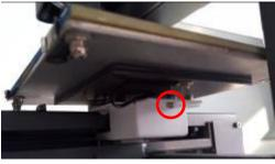
Notice: the platform may be adjusted repeatedly from 3.1.15 to 3.1.21 to ensure equal distance between the nozzle and the platform. Once confirmed, it does not need frequent adjustment.
