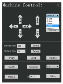
4.3.9.4 After movement to a position, to lock or unlock the motor, you can click "Lock" or "Unlock".
