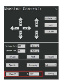
4.3.9.13 After a period of use, the height of the platform needs to be fine-tuned, you can directly modify the figure in the dialog after "Z:", and click "Setting".
