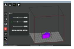
4.3.10.2 The imported model will be automatically placed in the center of the platform. You can move the slider in "X/Y/Z" with the mouse to change its position, and the model will move on the platform according
