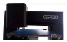
3.1.16 Click "START", the platform will move along the direction shown below. At this moment, you can observe the distance between the nozzle and the platform. If it is equal all the time, the platform has been leveled. Click "STOP" to stop the movement. If not, the platform needs to be debugged in accordance with the following steps.
