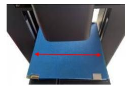
3.1.21 In the left and right movement, observe the distance between the nozzle and the platform. If it is equal all the time, enter the next step. If not, adjust the screw fixing the platform till it is equal.
