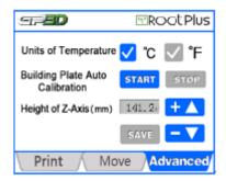
3.1.15 "Building Plate Auto Calibration" is the automatic detection of the platform. Press "Z+" in the interface "Move", and raise the platform to about 1mm from the nozzle.
