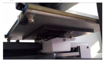
3.1.17 Click "X-" or "X+" to move the extruder to the central axis of the platform.
