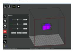
4.3.10.3 You can also directly input the moving distance in the slider dialog of "X/Y/Z". Notice: if the moving distance is beyond the maximum frame, the model will move to the position of the maximum frame, as shown below.
