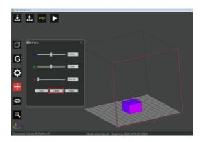
4.4.3 Click the left menu button to generate GCODE (PLA material used for printing), set the nozzle temperature at 220 °C and the platform temperature at 30 °C, and click "Setting", as shown below.
